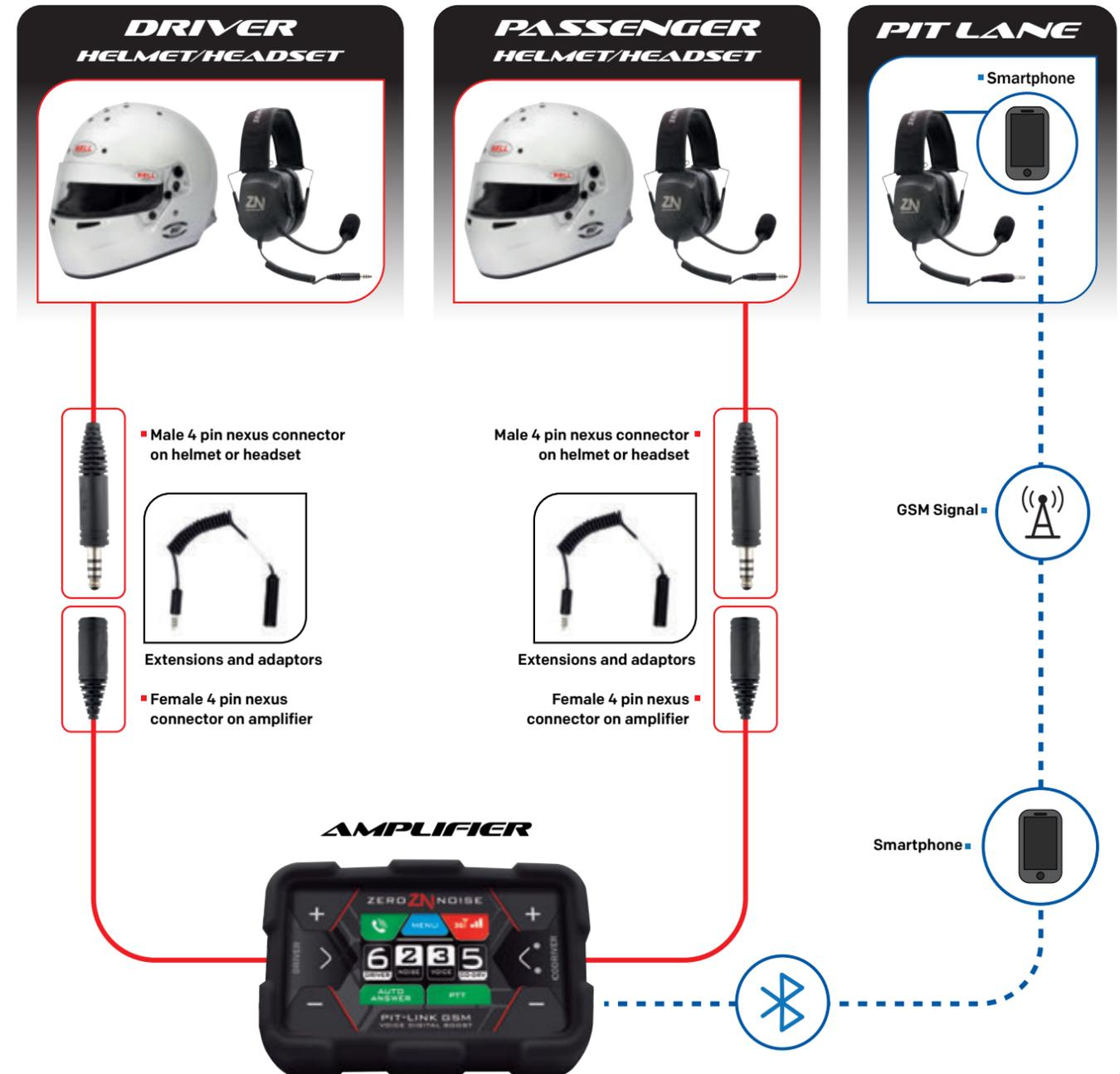
The Wired-Wireless (WW) System enables communication between driver and co-driver both in Wired and Wireless mode. When the helmet IS connected to the amplifier via cable, the communication works traditionally, also keeping compatibility with any Nexus communication system.
