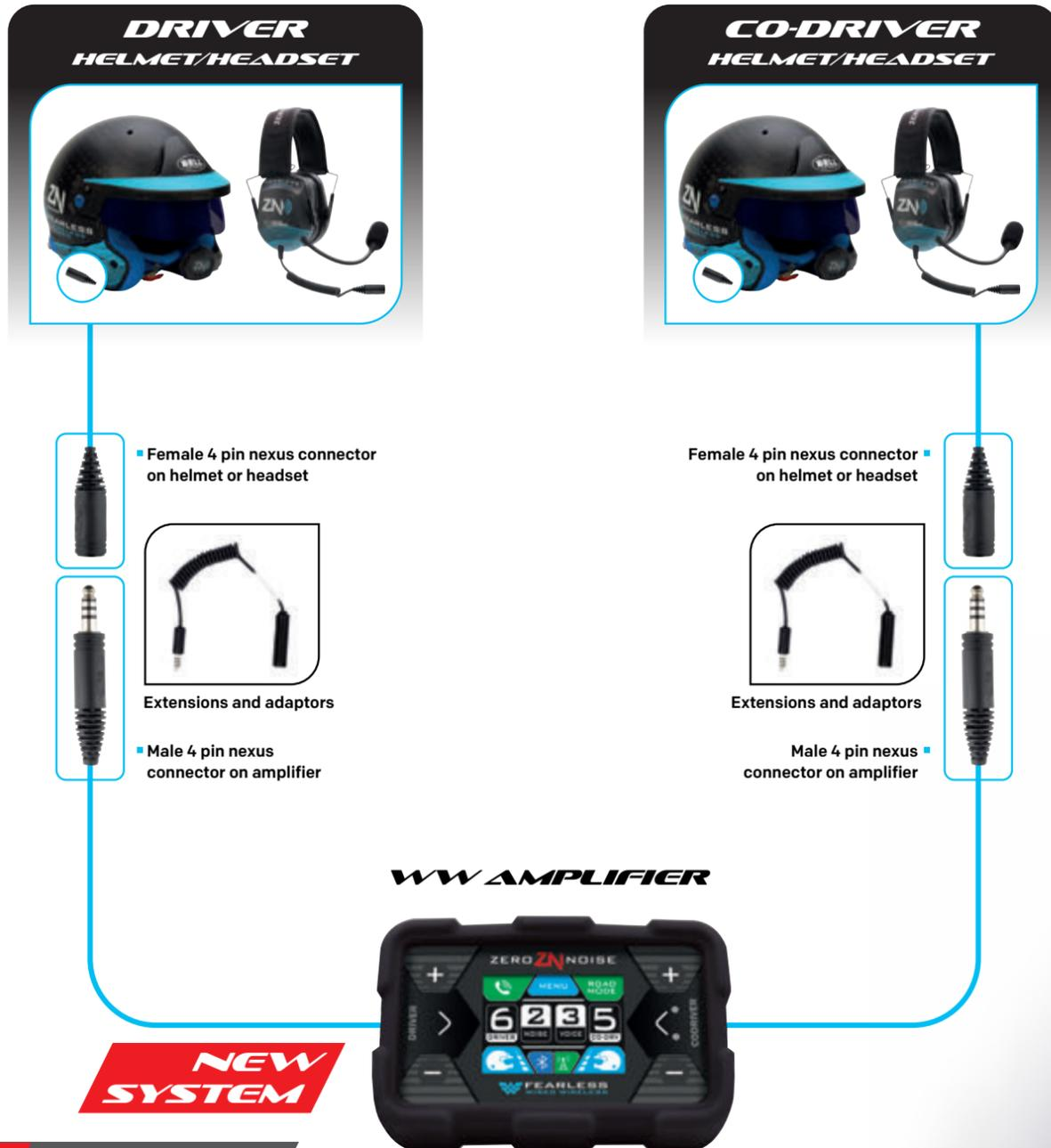
When the helmet IS NOT connected to the amplifier via cable, the system switches automatically to the wireless mode with no interruption whatsoever.
